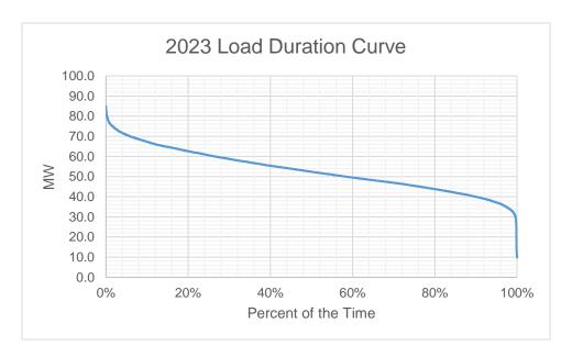
As shown in the above graph, the maximum load of the Company's power transformers in 2023 was 85.83 MW. Said maximum load did not include the requirement of the Company's 69 KV customers and the supply from embedded generators.
