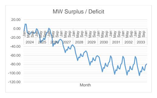
The graph above illustrates a supply deficit during certain periods. This deficit is primarily due to insufficient contracted capacity during peak hours. However, the overall supply has been sufficient to meet the Company's average demand in previous years.
