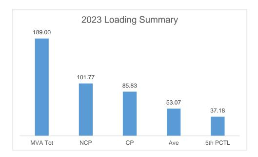
The Non-coincident Peak Demand is 101.77 MW, which is around 53.85% of the total substation capacity of 189 MVA. The ratio between the Average Load of 53.07 MW and the Non-coincident Peak Demand is 52.15%. A safe estimate of the true minimum load is the fifth percentile load of 37.18 MW which is 36.53% of the Non-coincident Peak Demand.
